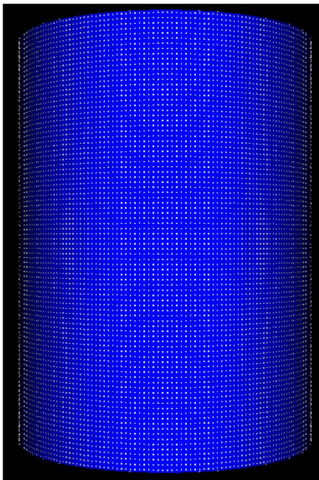
Figure 13: A Chroma rendering of the outside of the LBNE water Cherenkov detector. Blue indicates the opaque cavity liner, and the white dots are the back sides of the truncated PMTs poking through the sheet.
